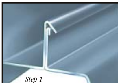
360 degree 3-stage "Pittsburgh" double lock seam
