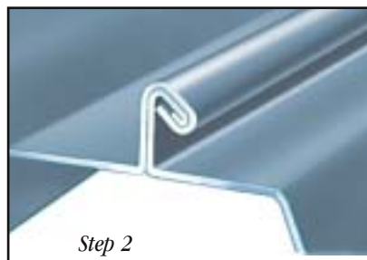
360 degree 3-stage "Pittsburgh" double lock seam
